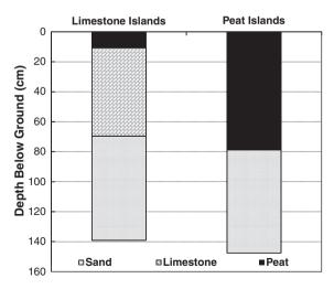
**Fig. 2.** The average below-ground depth (m) of sediment detected at the center of the peat and limestone tree islands when the groundwater wells were installed.
