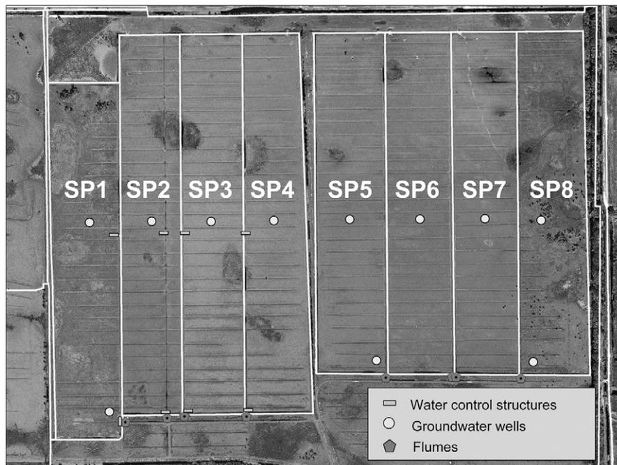
Fig. 2. Aerial image of the experimental pastures showing the location of the flumes, groundwater wells, and water control structures.
