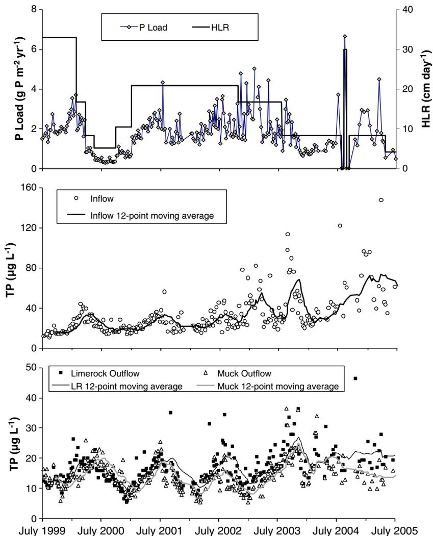
Fig. 2. Hydraulic loading rates (HLR) and phosphorus (P) mass loadings to mesocosms operated for 6 years on muck or limerock (LR) substrates. Inflow total P (TP) concentrations and outflow concentrations are shown as the average of duplicate mesocosms for each substrate. The moving average TP concentrations of 12 previous observations are also shown.
