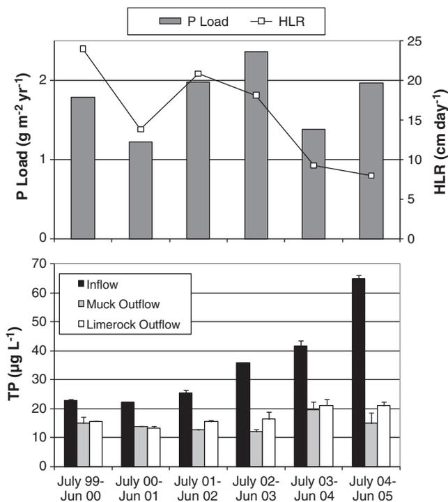
Fig. 3. Annual phosphorus (P) loading, hydraulic loading rate (HLR), and inflow and outflow total P (TP) concentrations of duplicate mesocosms operated on muck or limerock substrates for 6 years. The error bars represent  $+1$  S.D. of the mean of duplicate mesocosms.
