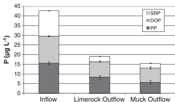
**Fig. 4.** Mean ( $\pm 1$  S.D.) concentrations of phosphorus (P) species for duplicate mesocosms operated on muck or limerock substrates collected during the final 3 years (June 2002–June 2005) of the study.
