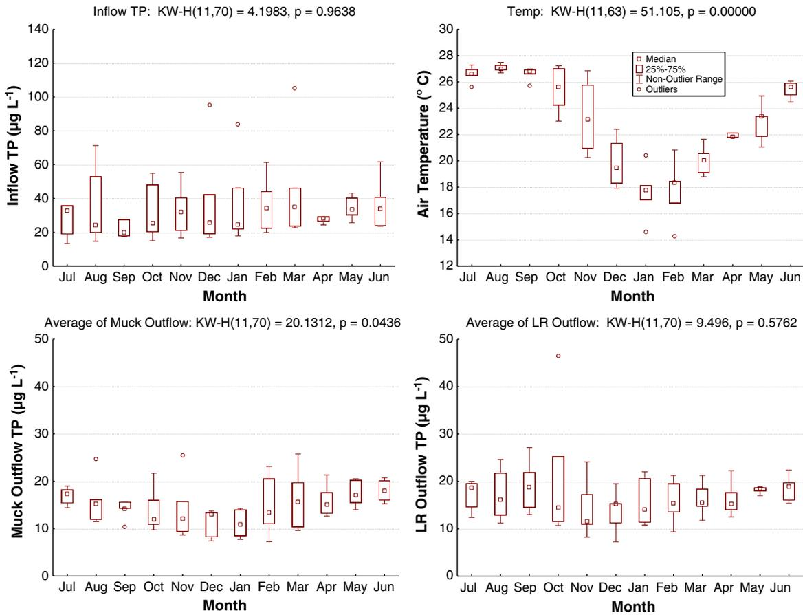
**Fig. 7.** Seasonal trends in air temperature and total phosphorus (TP) concentrations in mesocosm inflow and outflow surface waters over the period of record. Values are derived from monthly averages across 6 years for duplicate mesocosms on limerock or muck substrates. Air temperature data from the South Florida Water Management District was recorded at station ENR308, ~2.7 km north of the mesocosm facility.
