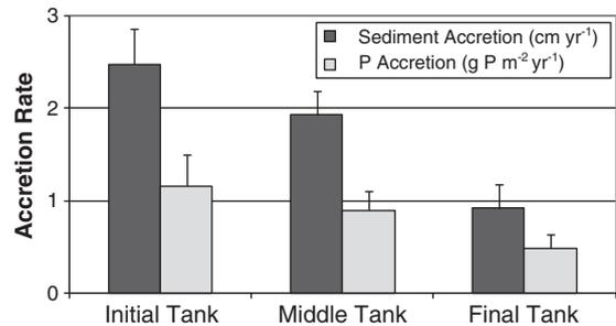
**Fig. 8.** Mean (+1 S.D.) sediment and P accretion rates from each tank-in-series along the flow-path for duplicate mesocosms operated on muck substrates. Sediment was collected on December 15, 2004, after the mesocosms had been operational for 5.5 years.
