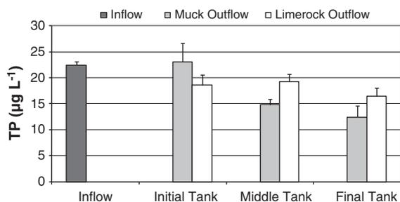
**Fig. 5.** Mean ( $\pm 1$  S.D.) total phosphorus (TP) concentrations at the inflow to the mesocosm and outflow from each tank-in-series along the flow path for duplicate mesocosms with muck or limerock substrates. Data were collected during a 3-month period from August 2001–November 2001.
