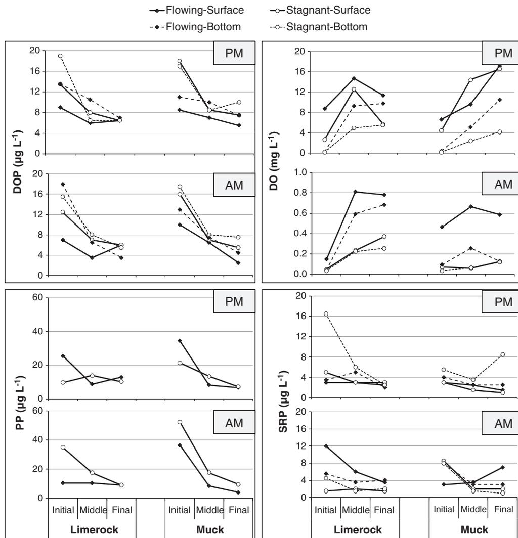
**Fig. 6.** Diel surface and bottom water dissolved organic P (DOP), particulate P (PP), soluble reactive P (SRP) and dissolved oxygen (DO) concentrations from each mesocosm-in-series along the flow path for duplicate mesocosms operated on muck or limerock substrates. Samples were collected during flowing conditions (7/29/04) and at the end of a three-week stagnant period (8/17/04). Bottom water PP was not measured.
