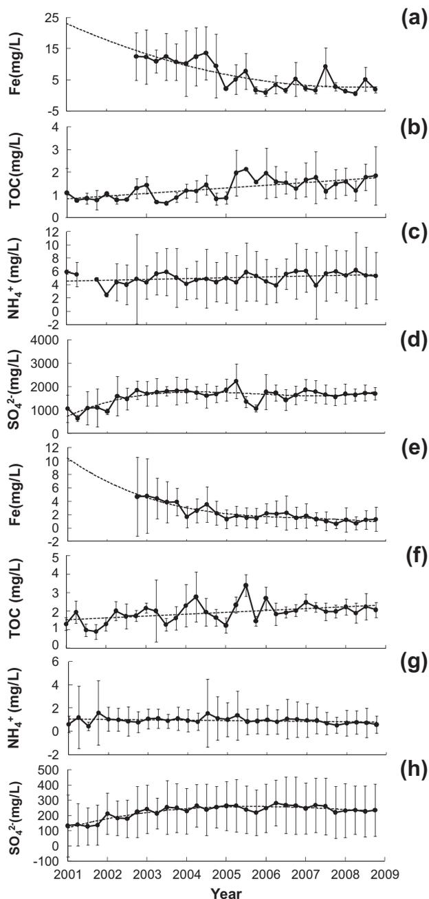
Fig. 7. Seasonal variations of average Fe, TOC,  $\text{NH}_4^+$ , and  $\text{SO}_4^{2-}$  concentrations in saline wells (a–d) and non-saline wells (e–h). The dashed lines denote the linear or polynomial regressions of explanatory variables. Error bars represent standard deviation from mean of variables.
