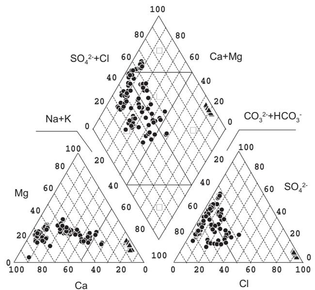
Fig. 6. Piper diagram of 8-years groundwater quality data of 10 monitoring wells. Solid triangles (▲) and circles (●) denote saline wells (Nos. 1 and 10) and non-saline wells (Nos. 2–9), respectively.
