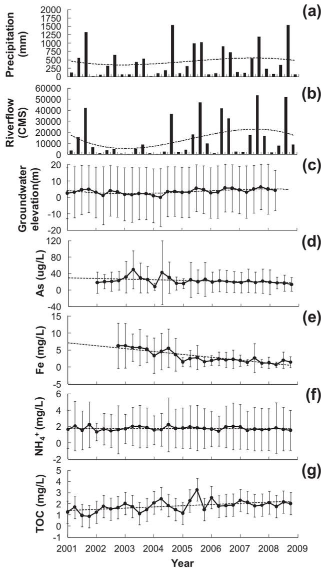
**Fig. 2.** Seasonal variations of the hydrological and geochemical explanatory variables during 2001–2008. (a) precipitation from a weather station, (b) river flow records from a river flow gauging station, and average (c) groundwater elevation, (d) As, (e) Fe, (f) TOC, (g)  $\text{NH}_4^+$  of 10 shallow wells. The dashed lines denote the linear or polynomial regressions of explanatory variables. Error bars represent standard deviation from mean of variables.
