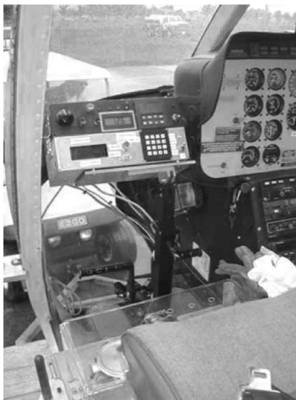
Figure 3. The Airborne Height Finder (AHF) installation. The AHF is positioned on the left-hand side of the helicopter in front of the AHF operator and the global positioning system (GPS) containing the flight line information is positioned on top of the instrument console where it is visible to both the pilot and the AHF operator. The AHF plumb-bob and calibration plate are mounted outside the helicopter door.
